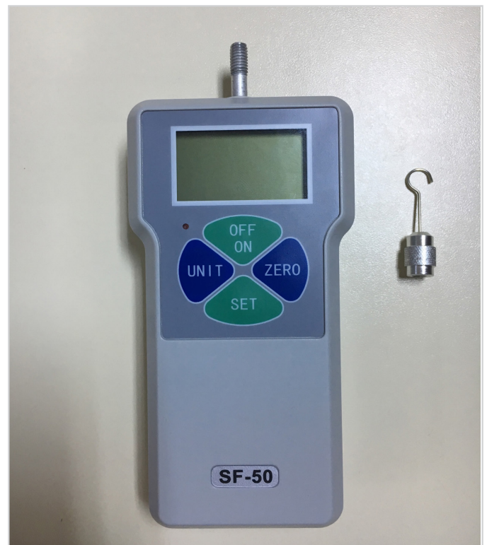
Figure 3. Digital Newton-meter that was used for measurements
